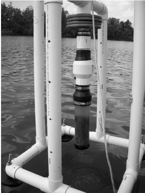
**Figure 2.** Modified HYPOX (see Gardner et al., 2009) sampler used to collect sediment cores from Lake Wister for sediment O<sub>2</sub> demand and P release rates, as measured in the laboratory.
