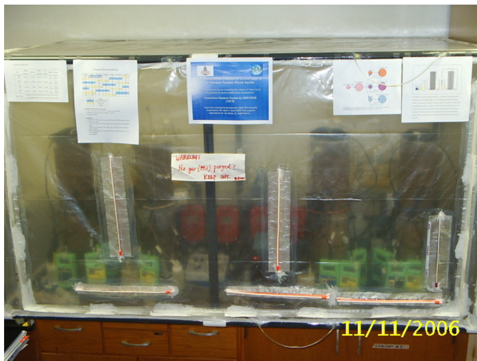
(b) Outside shielding box filled with nitrogen gas 99.9%.
